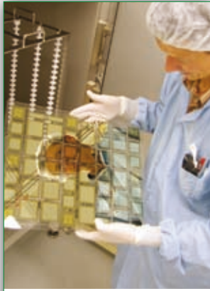
Inspection of OLED Lighting panels during pre-pilot production in Aachen Courtesy: Philips Lighting
