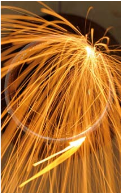
Fig. 4.2.12 Single-sided tube cutting with fibre laser © TWI Ltd
