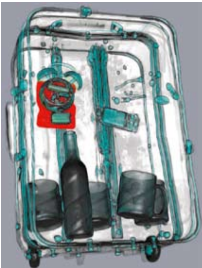
Fig. 4.5.6 X-ray baggage checks are used to detect prohibited items © Sagem
