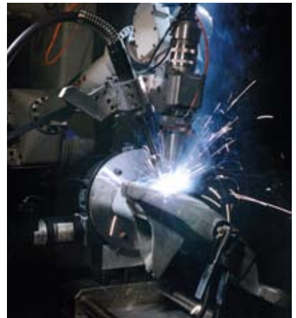
Fig. 4.2.5 Hybrid laser-arc welding of an aluminium axle © TWI Ltd
