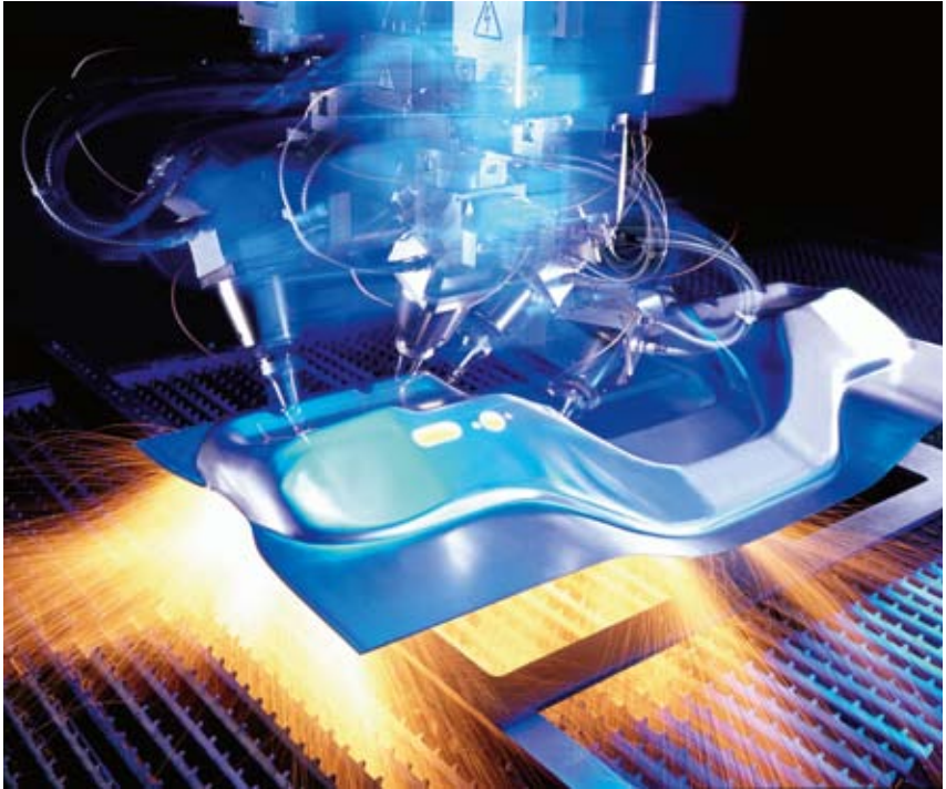
Fig. 2.3.3 Laser processing system for cutting and welding © TRUMPF GmbH + Co. KG
