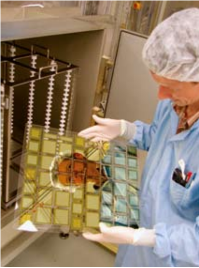
Fig 4.4.23 Visual inspection during OLED pilot production in Aachen, Germany © Philips
