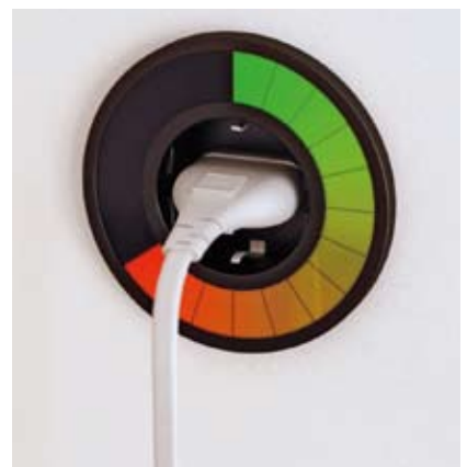
Fig. 4.4.24 Electrowetting displays make new applications possible, like this socket power meter © Liquavista & Daan Pothoven
