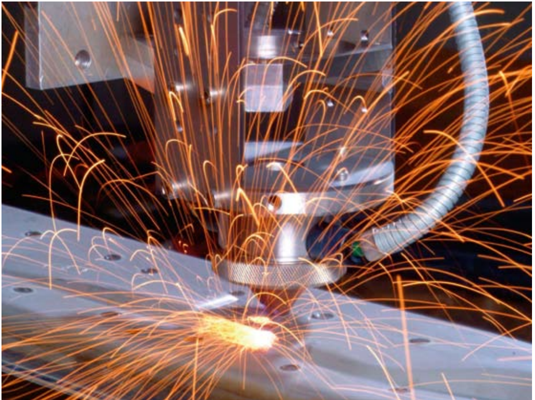
Fig. 4.2.14 Cutting and welding an automotive component with a laser combination head in one setup © Fraunhofer-Institut für Lasertechnik
