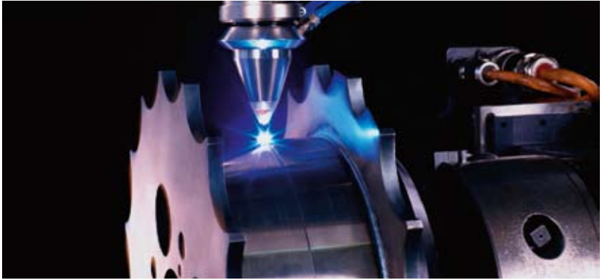
Fig. 4.2.4 Laser welding with a TruFlow laser © TRUMPF GmbH + Co. KG
