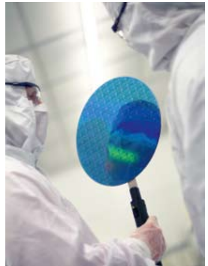
Fig. 4.6.2 A silicon wafer © IMEC
