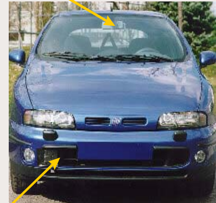
LIDAR (ON THE RIGHT TO RECOGNIZE VEHICLES ALSO IN THE RIGHT LANE DURING THE LANE CHANGE PHASE)
